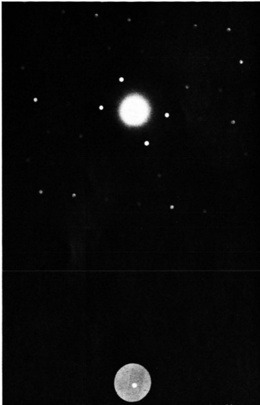
Fig. 2. Shadow image of part of a rectorite crystal and its diffraction pattern. The bright spot locates the diffracting area exactly.
